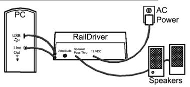
The following steps are required to enable the RailDriver internal subwoofer. Power and audio connections are not required for operation of the RailDriver controls, but they do enhance the driving experience.
