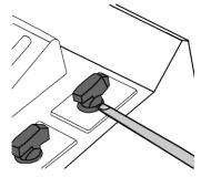
To remove wiper and light switch caps for labeling, insert a thin bladed screwdriver into the slot on either side of the switch and carefully pry up until the switch cap pops off.
